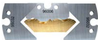
Profile soffit moulding, 70 mm
