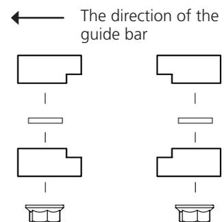
**!** The slide rails have to be assembled as in illustration B when the saw carriage is equipped with crank and bar nose steering.
