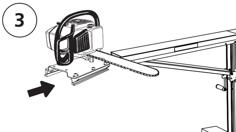
Push the carriage onto the guide rail with the guide bar in the direction of the log beds.
