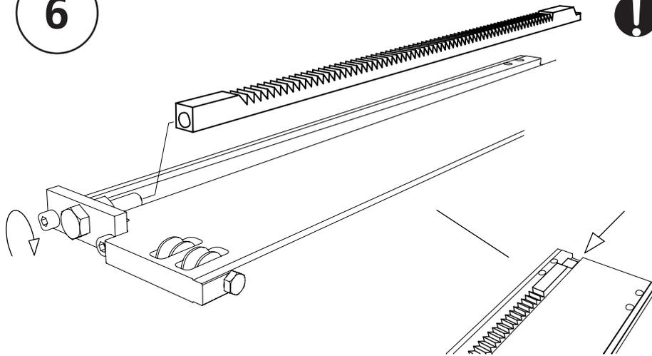
**!** Make sure that the end of the ratchet bar does not extend over the end of the lifting beam, since this makes it impossible to assemble the log bed. The ratchet bar is normally slightly bent towards the toothed side. When screwing it into place, it will get a tight fit against the lifting beam by the tension created.
