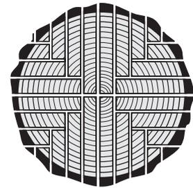
Start by cutting the log in half at its centre. Then you cut through the middle of the halves to get quarters.
