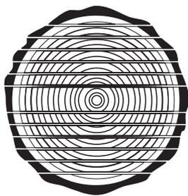
When you are going to slice up a log, it is best if you first cut off a thin slab and then turn that side down to make the log rest on a flat surface on at least one of the log beds. This prevents the log from moving
