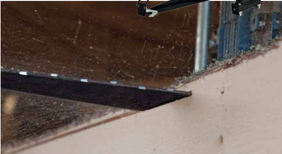
• Just in time for the sawing season Logosol launches a faster electric saw head for the Logosol Sawmill. The biggest novelty for the user is a special guide bar for rip sawing that gives a finer sawn surface.
