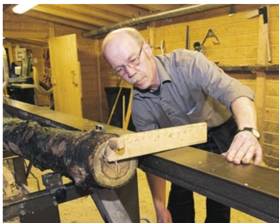
Pelle Boström, Sweden, demonstrates how the setting gauge works. When it lies like this on the guide rail, the sawn surface will be exactly where the nail is fastened.
