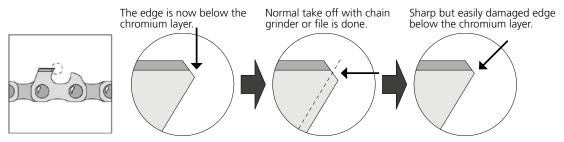
the next time you sharpen the chain. The chain may get sharp, but because the new edge is not in the chromium layer it will very quickly become dull and, in the worst case, overheat again. To repair the damage, you have to file off a lot of the cutter.
