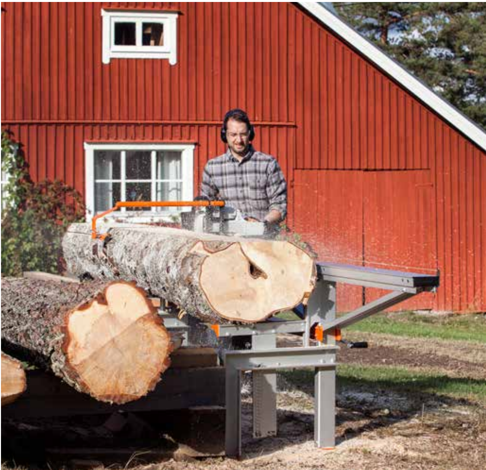
• The Logosol F2 can easily handle logs that are up to 60 cm in diameter. Winches are used to lift the logs up so you can work upright most of the time.
