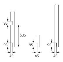
**1.** Start by sawing the boards for the barbell rack and sawing the recesses on the standing posts according to the measurements above. Then screw them together as shown.
