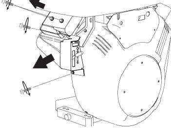
Release the throttle cable bracket on the front of the engine, then remove the end of the cable from its bracket. This task is easier if you use pliers to remove the end of the cable.
