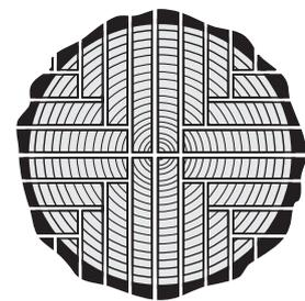
Start by cutting the log in half at its centre. Then you cut through the middle of the halves to get quarters.
