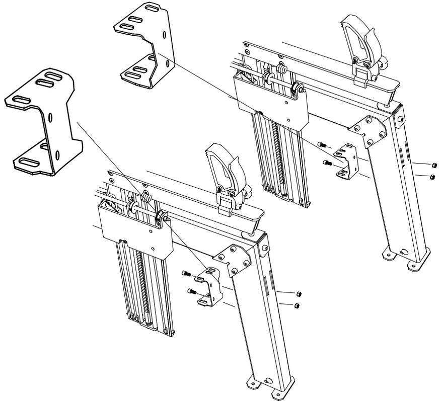
Installing horizontal strut mounts for a 5 m long guide rail. Note in which direction each mount is fitted.
