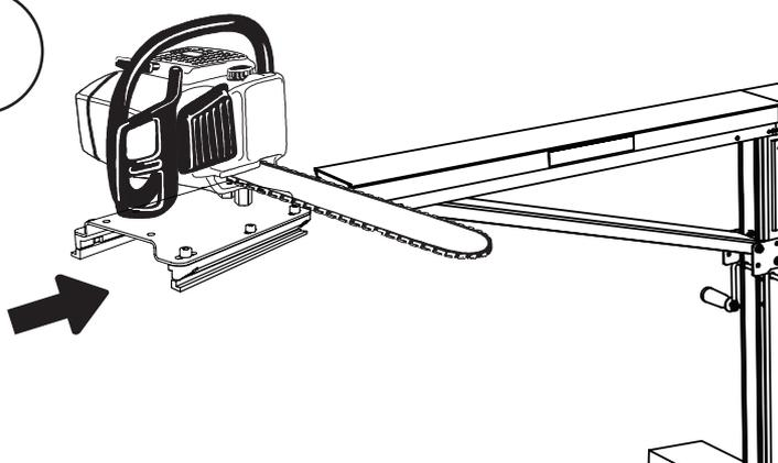
Push the carriage onto the guide rail with the guide bar in the direction of the log beds.
