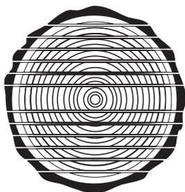
When you are going to slice up a log, it is best if you first cut off a thin slab and then turn that side down to make the log rest on a flat surface on at least one
