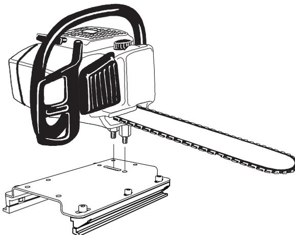
Fit the Logosol nuts through the track in the carriage. Tighten the chainsaw into place by using the chainsaw's guide bar nuts under the plate.
