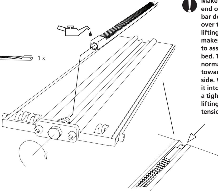
**!** Make sure that the end of the ratchet bar does not extend over the end of the lifting beam, since this makes it impossible to assemble the log bed. The ratchet bar is normally slightly bent towards the toothed side. When screwing it into place, it will get a tight fit against the lifting beam by the tension created.
