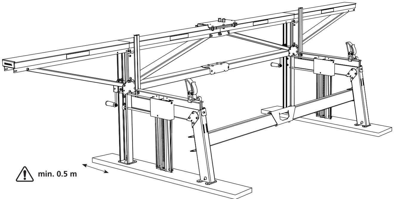
When the sawmill is placed directly on the ground, the surface must be firm and level enough to drive a regular passenger car on.
