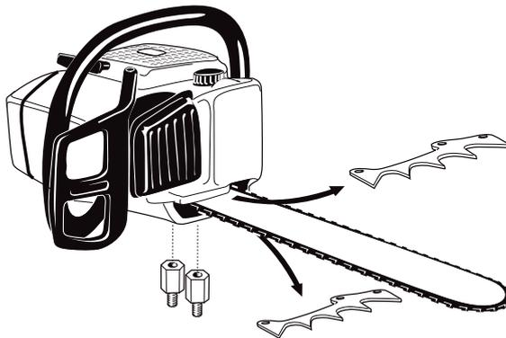
Unscrew the two guide bar nuts from the chainsaw and remove the guide bar cover.
