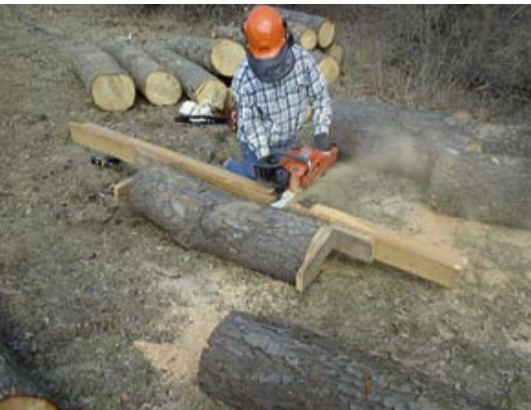
Ted Christiansen, March 2006: " Milled some cherry, ash and pine logs yesterday. Since the logs were all about 14" diameter 4 footers, we split them in half first using the Timberjig. They will be milled into boards using a Jet 18" 3HP vertical bandsaw with milling sled. First cut using 16" bar."
