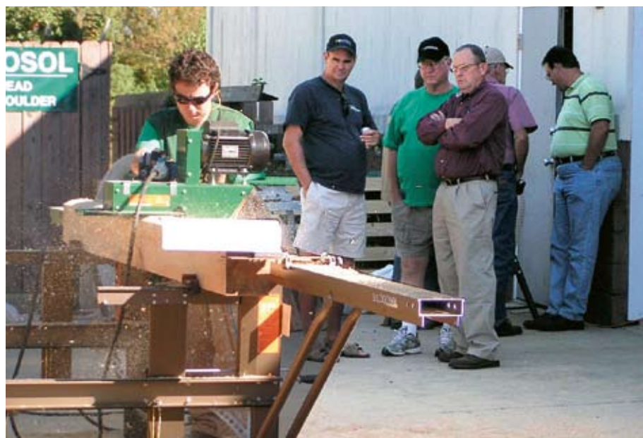
Rivers Griffin demonstrates how to use the M7 sawmill to make log house facing.
