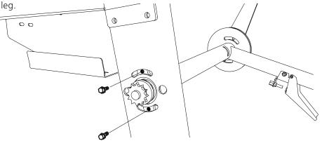
Secure the tube handle with the long fixing bolts. Note that the inner nut should be placed so that the head of the Allen bolt is flush with the surface of the carriage leg.
