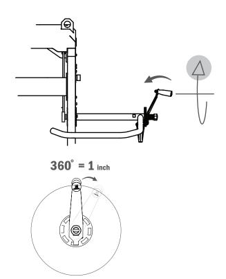
The locking mechanism of the crank is divided in eight steps per revolution. Each step moves the sawhead by 1/8 inch, and one full revolution represents 1 inch. A disc with 16 steps is available as an accessory.
