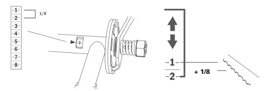
On the crank shaft, there is an opening where you can see numbers on a scale. This scale has eight steps, where each step is 1/8". **TIP:** When a board is cut above the blade, you have to compensate for the kerf, i.e. 1/8". The wood piece below the blade never needs to be kerf compensated. It has the same measurement as the one shown on the absolute scale on the front leg of the carraige.
