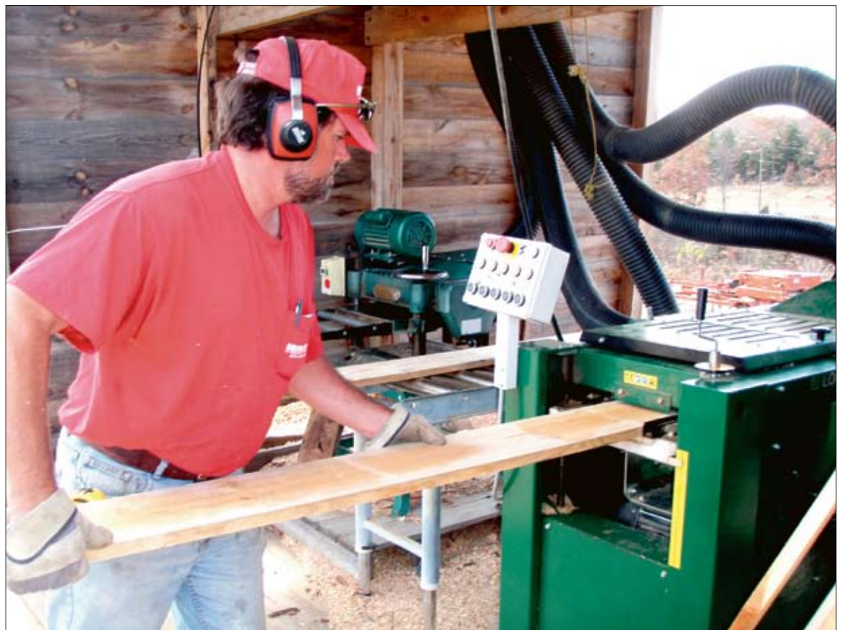
Dave Barnes feeds another board through his Logosol PH260 for surfacing on all four faces.
