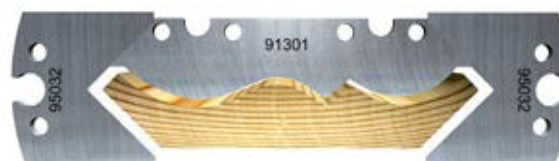
Swan neck soffit moulding, 120 mm
