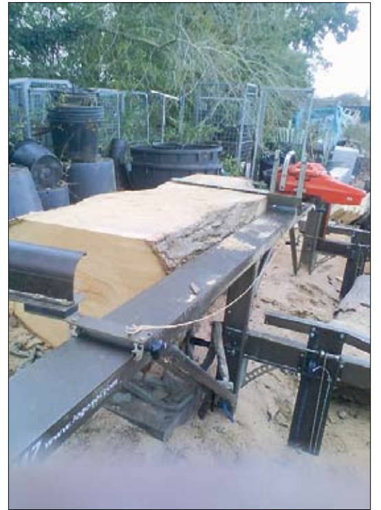
M7-owner Dave Ellis blocking up his log to the correct height with a chainsaw before he uses his Logosol M7.
