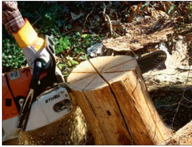
First 4 chainsaw cuts are made vertically in a short standing log to within 4" of the base.
