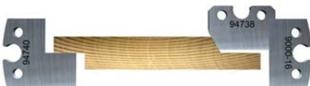
Double rabbet 60° chamfer
