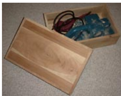
Cherry box for belt sander. Dovetailed with figured floating panel lid
