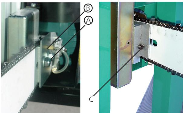
The “shortness” of a new chain may make fitting it around the sprocket difficult. Chains stretch with use and are then easier to fit.
