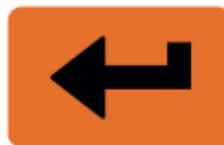
The **Enter button** is responsible for saving the setting or entering the command to position sawhead to the next cutting place taking into account kerf, etc.
