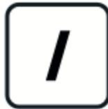
Pressing the divide button followed by a numerical value and then pressing enter will create a board list, based on the height where the sawblade is located, and where each board is of the specified thickness, taking into account the kerf thickness.
