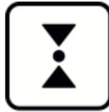
The "**remember the height**" or "**remember the point**" button plays a crucial role in setting the starting point for sawing logs on the sawmill bed. It is recommended to use this button only for the first cut after placing a new log on the sawtable.
