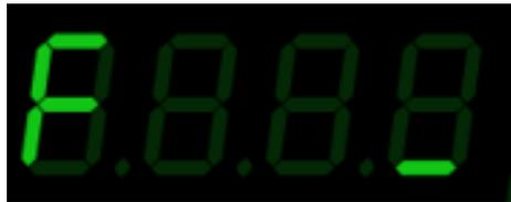
Then enter the number of the settings and press Enter button. If this is an important setting, then the system will require a code (done so that the sawmill operator cannot change the settings uncontrollably), see fig. below.
