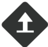
The "Bump up" button has two main functions. Firstly, it allows for upward movement of the sawhead within the designated limits set by the "virtual" upper limit switch (F 88). This feature helps to prevent accidental damage to the sawmill equipment and ensures safe operation.
