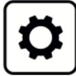
The settings (or menu) button is responsible for entering the menu and setting new system parameters. To enter the "settings menu" long press this button until you see F on the display. In case you see CodE then you need to enter Code for entering the settings
