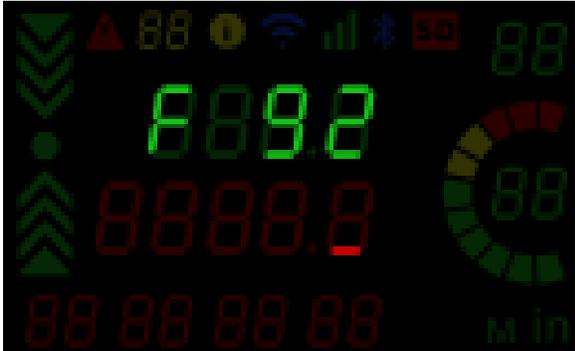
2. Enter the measured distance in p.1 and press Enter button. Then F98 will display.
