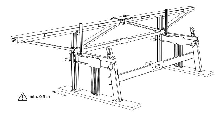
When the sawmill is placed directly on the ground, the surface must be firm and level enough to drive a regular passenger car on.
