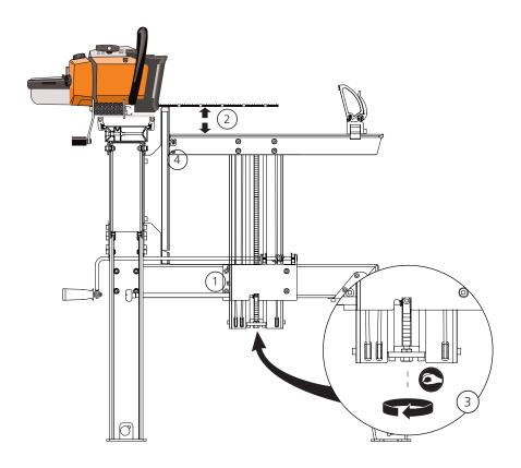
When the log lifter is being cranked down, check that it moves easily through the ratchet cam housing driven by its own weight.
