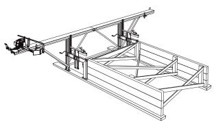
Example of a log table for longterm set-up. Log ladders of steel are available as accessories for the Logosol F2+.
