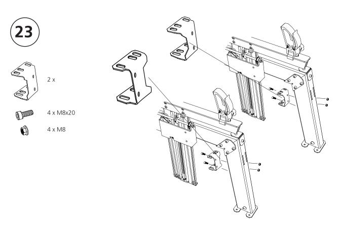
Installing horizontal strut mounts for a 5 m long guide rail. Note in which direction each mount is fitted.
