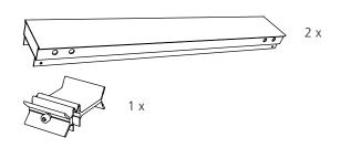
The joint coupler should be fitted in the guide rail with its opening facing up, as in the illustration. The lock nut should be positioned correctly in the nut recess. The bolt should not be tightened when the joint coupler is installed in the guide rail ends.
