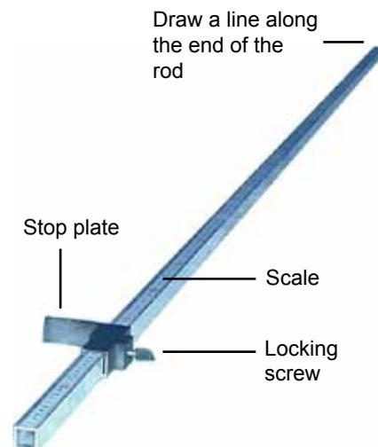
Using the measuring stick, measure out and draw the lines for the next cut. Position *Stack Cutter* and repeat the cutting procedure.
