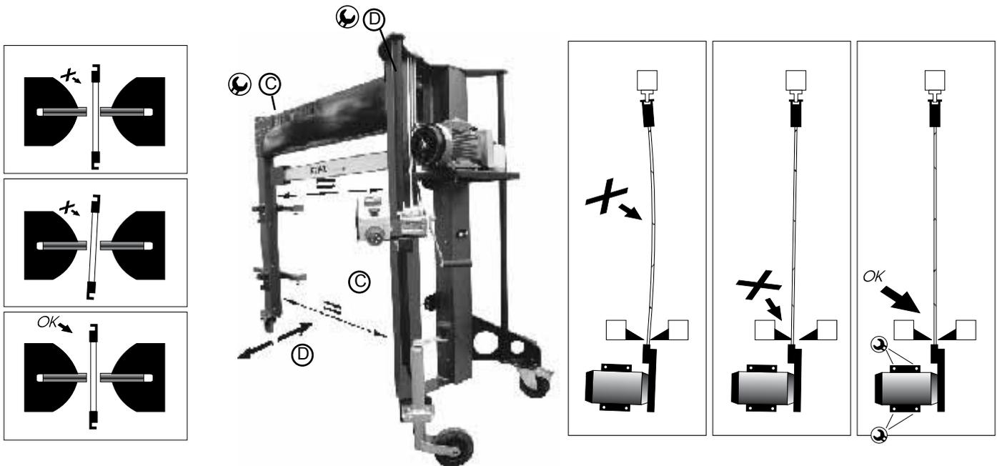
Schematic sketches of the machine's sighting rod on the motor side and the saw unit seen from above. "⊗" shows incorrect adjustment, "OK" shows correct adjustment. This symbol "→" shows where to adjust.
