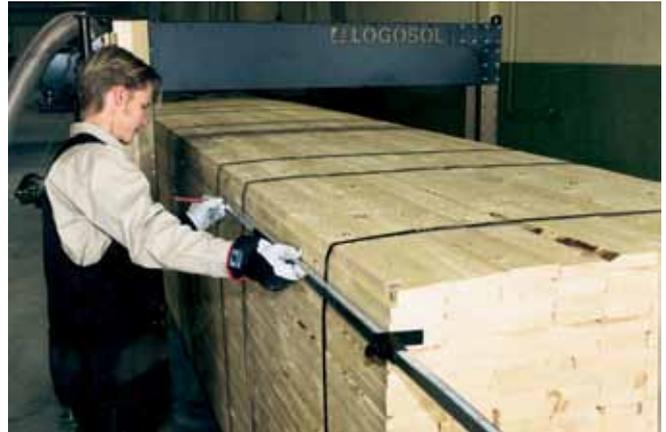
At the top and the bottom of both sides of the stack, set the stop plate against the cut surface and mark the end of the rod.
