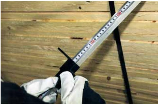
Set the measuring stick's stop plate to the desired length.
