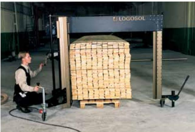
3. Align the upper sight exactly with the line. On the side that is not going to be cut off, fix a screw into the stack through the hole in the sight.
