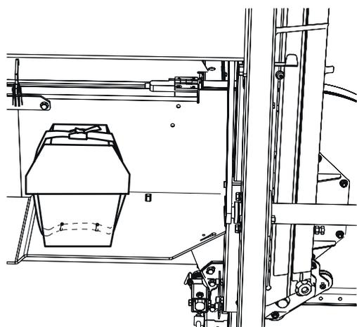
The battery is placed in the protective box and secured using the strap as illustrated.
