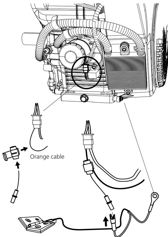
**11** Now connect the battery to the motor according to the sketch.
