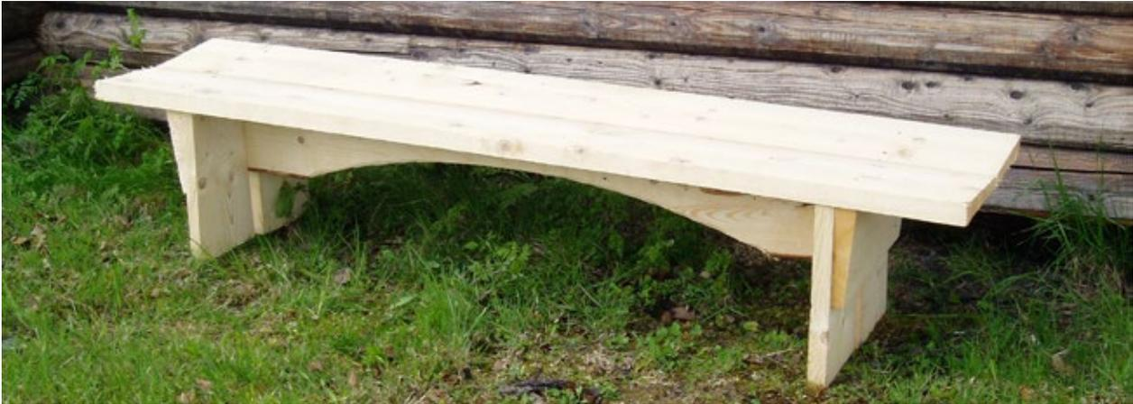
The transformation from raw timber to a finished bench takes around an hour. Use a chainsaw, a yardstick, a carpenter's square, a hammer, and nails. No need to be a nervous Nelly - it will turn out just fine!
