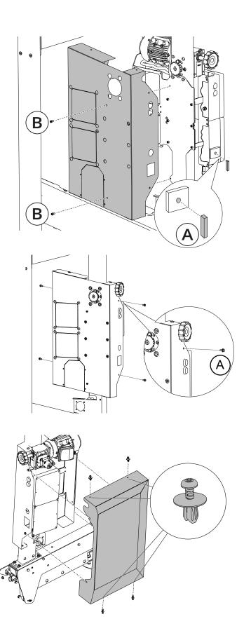
Slide the electronics cabinet's front cover under the four bolts installed under item 39. Tighten the four bolts. Press in the four quarter-turn fasteners and tighten the bolts.
