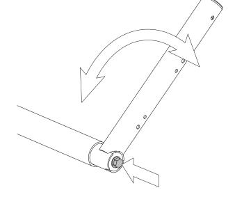
Loosen the lower tubular arm bolts. Adjust the arm to the desired height. Then tighten the bolts.
