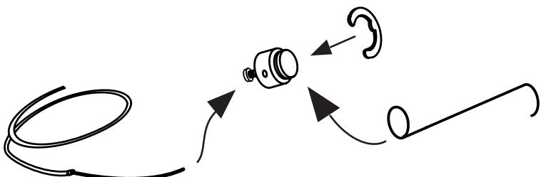
Fit the throttle link on the cable retainer, then lock the assembly into position using the lock washer.
