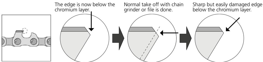
the next time you sharpen the chain. The chain may get sharp, but because the new edge is not in the chromium layer it will very quickly become dull and, in the worst case, overheat again. To repair the damage, you have to file off a lot of the cutter.
