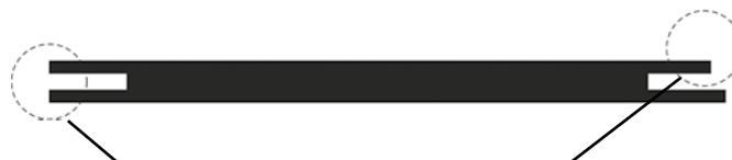
Unevenly worn bar rails can mean that the bar is not fitted straight in the bar attachment. It is normal that the lower bar rail is worn slightly quicker due to the round shape of the log.
