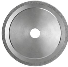
The diamond grinding disc is especially suitable for sharpening ripping chains, since they only need to be ground off a little. If you avoid using the diamond grinding disc for heavy sharpening of e.g. cross-cutting chains that have cut in stone, the life of the diamond grinding disc will be very long.
