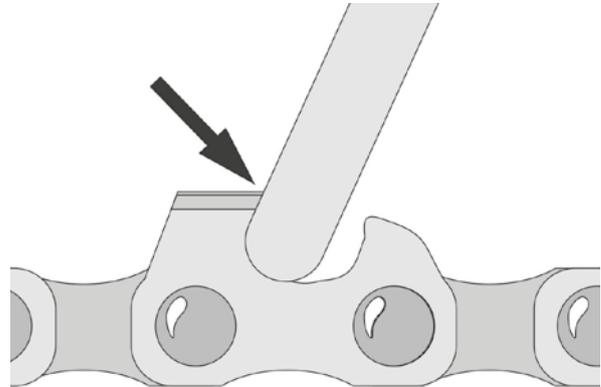
*It is important that the edge is sharpened with a tool surface that is free from grindings.*
