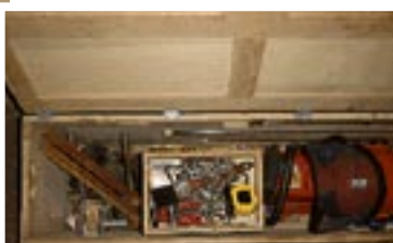
Cherry box for belt sander. Dovetailed with figured floating panel lid
