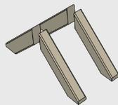
**5.** Screw or nail the legs to two of the ends.
