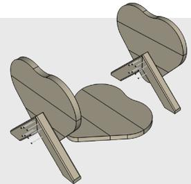
**6.** Nail the hearts to the joist. Start with the one in the middle at the top.
