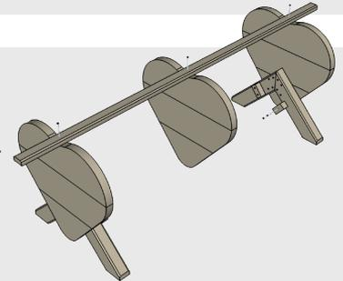
**7.** Continue with the rest of the joists. By the legs you might need extra pieces to fasten the joists.
