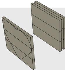
**3.** Cut out the shape with a band saw or jigsaw. Use it as a template for the other two ends and cut these out as well.
