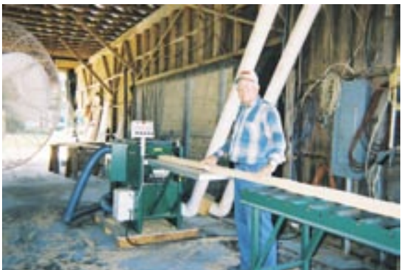
That is me feeding 2 x4 into my PH260. I have done quite a bit of 2 in lumber. I did a custom job of over 10 thousand board ft. of mostly 2 x 10. The customer built a house with it and was well pleased. The PH260 handled the job very well.
