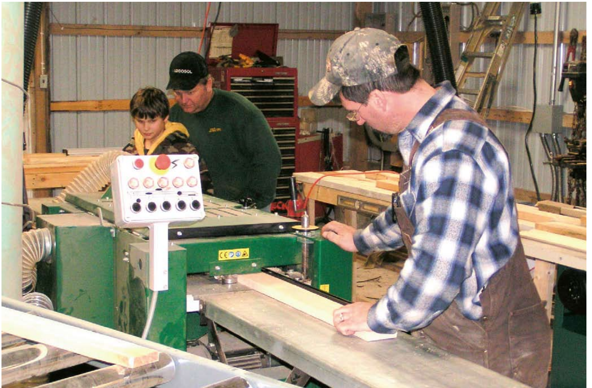
John Arnett (right) puts a board through the PH260 to test the knife settings. His brother Ron (center) and nephew Zach watch the outfeed.
