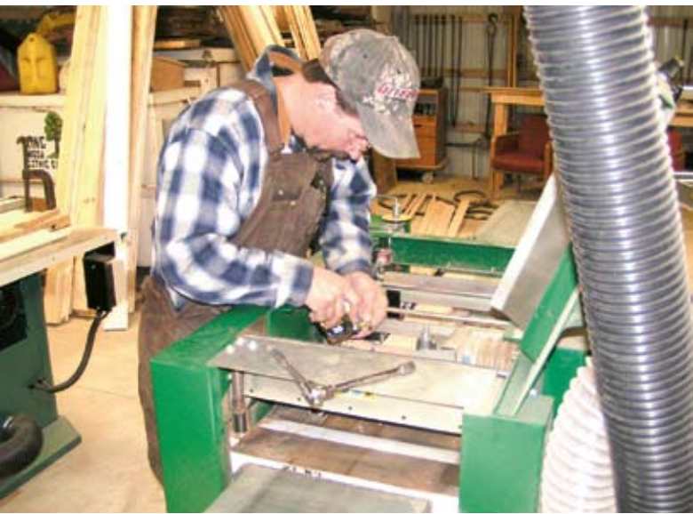
John Arnett installs a set of knives for a new trim pattern. He says it takes about thirty minutes to change the knives.
