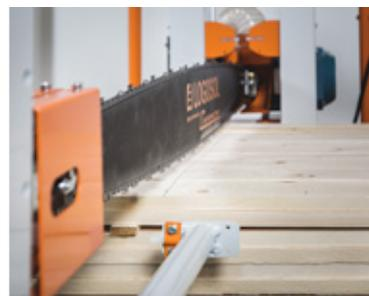
The guide bar, which is guided at the bar nose, cuts linearly vertically.
