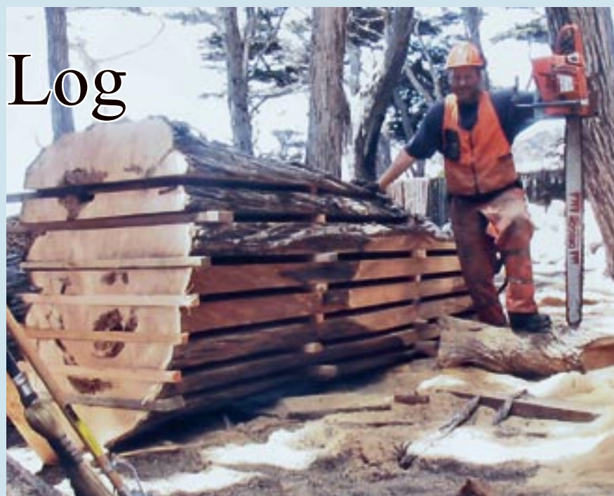
Rob next to California Cyprus log stacked to dry in original log shape Japanese style, log cut using the M-7 in inversion fashion
