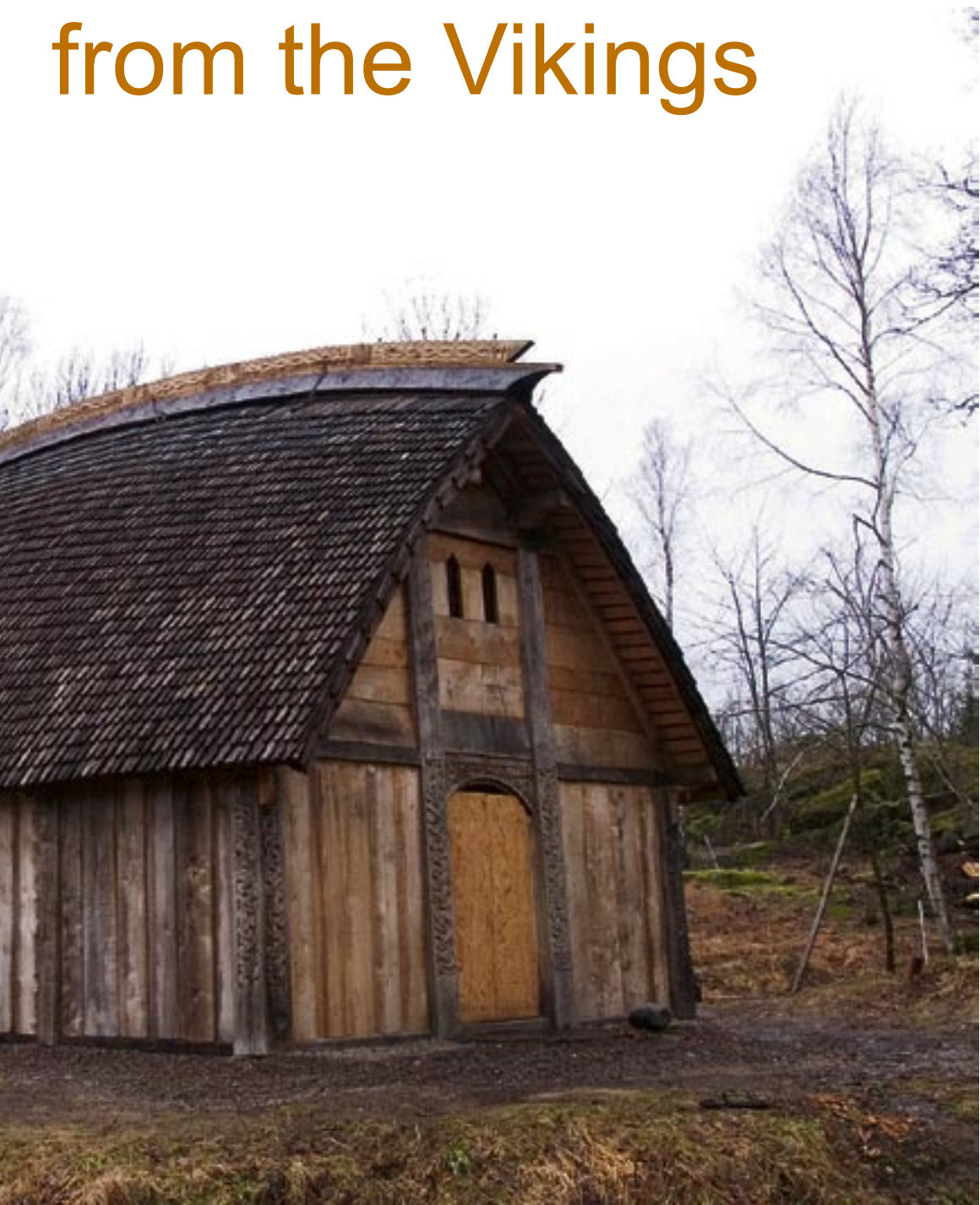
The Viking village is built on the Danish model. A house for a king or one of his closest men. The house has a well thought-out shape with its dome-shaped walls and roof. It gives the house good ventilation and takes out the smoke from the hearth without the house having a chimney.
