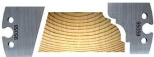
Lower window lining, Villa Frimodig
