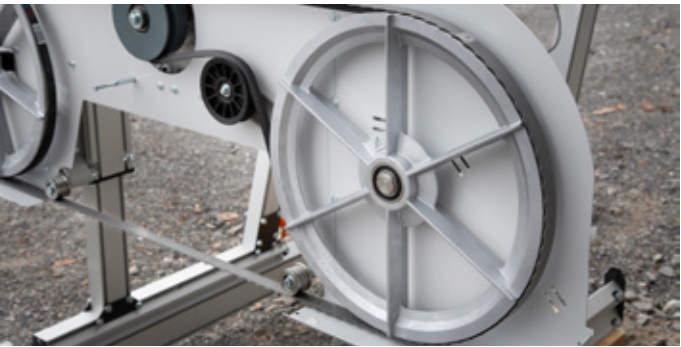
Band wheels with fan blades, cools the blade and keeps the cover clean.
