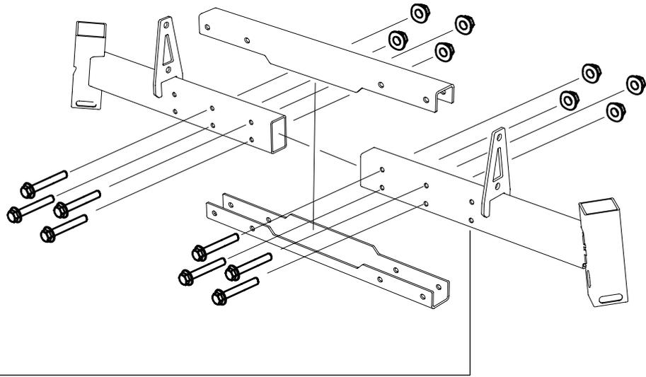
The inner row of holes is to be used on B751 Pro.
