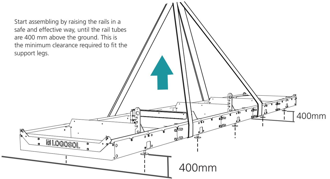
Recommended positions of the support legs on the rail frame.
