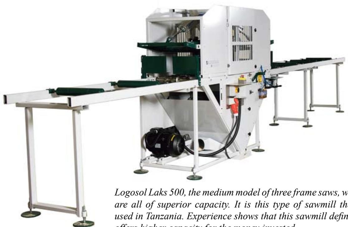
*Logosol Laks 500, the medium model of three frame saws, which are all of superior capacity. It is this type of sawmill that is used in Tanzania. Experience shows that this sawmill definitely offers higher capacity for the money invested.*
