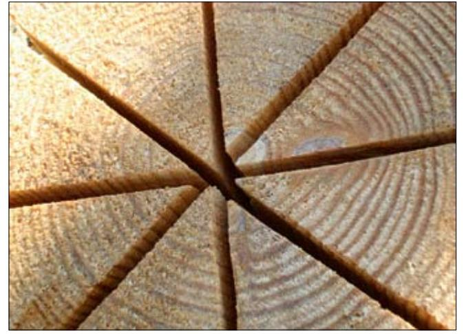
First 4 chainsaw cuts are made vertically in a short standing log to within 4" of the base.
