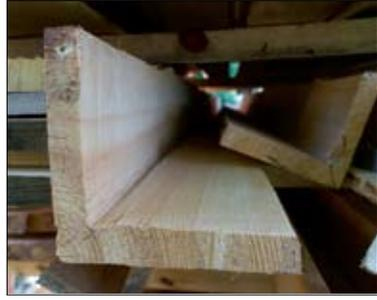
Wedge-shaped and wide siding boards are sought-after products.
