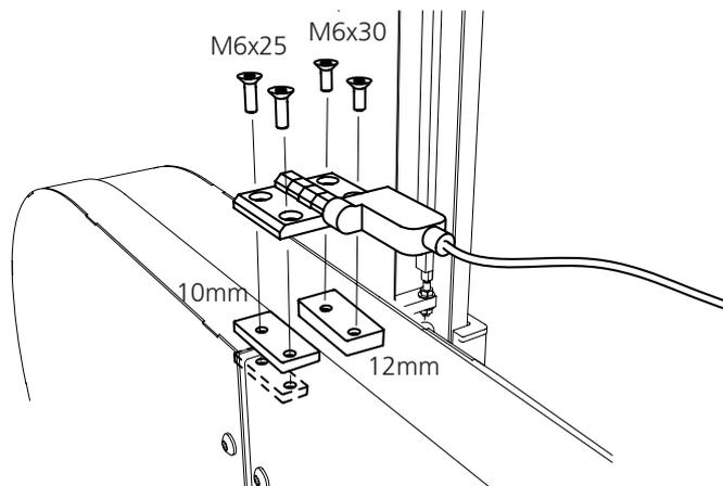
**13** Now connect the safety switch to the engine as illustrated.
