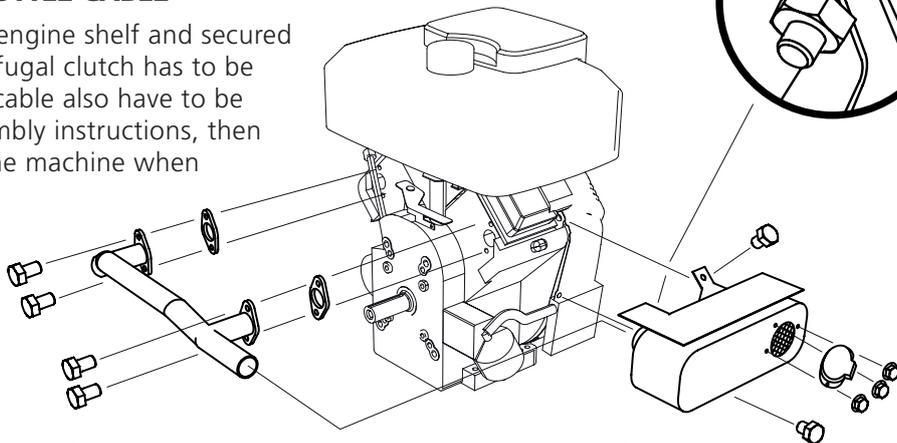
**2** Install the engine on the engine shelf: Install the engine on the saw head before placing the saw head on the rail. Two people are always required to help when the engine is lifted into place. The illustration below shows the hole pattern for installing the 18 and 23 hp Briggs engines, respectively.
