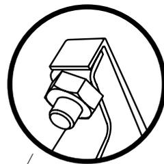
**1** Fit the manifold and the silencer on the engine.
