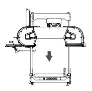
Tip: Work with the sawhead lowered to its lowest position to facilitate access to the engine.
