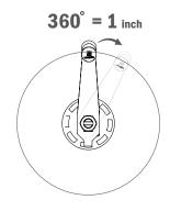
The locking mechanism of the crank is divided in eight steps per revolution. Each step moves the sawhead by 1/8", and one full revolution represents 1".
