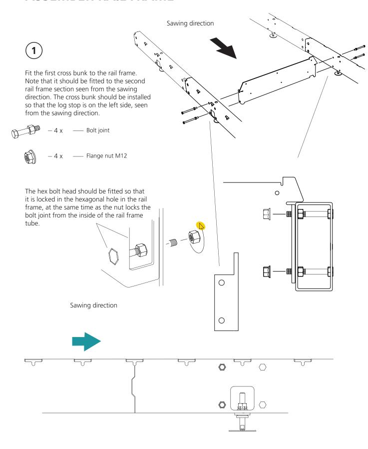
Install the other cross bunks as shown in the illustration. Note that the first rail frame section, seen from the sawing direction, should not have a cross bunk. This is because that section lies outside the effective sawing length.
