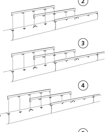
The last short rail section should be fitted the same way as the first one. See the first step of assembly on page 36.
