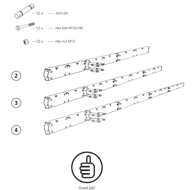
Repeat the assembly steps for making the other rail frame side.
