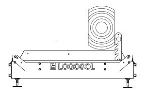
Rotate the log 90° so that one of the freshly sawn sides rests flat against the log supports, and then clamp the log in position.
