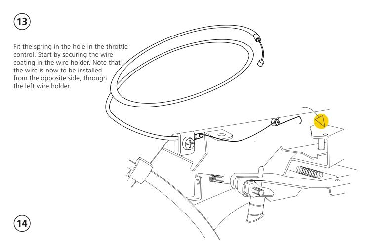
Tighten the wire until full throttle on the handle gives full throttle on the engine.
