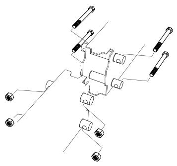
Secure the bolt joints. Ensure that the joint between the rail frame sections stays straight when tightening the bolt joints.
