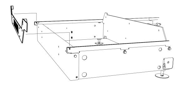
Secure the bed end frames with bolts and nuts.
