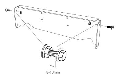
Fit the end plate to the end of one of the rail frame sides, then repeat this at the end of the other rail frame side.
