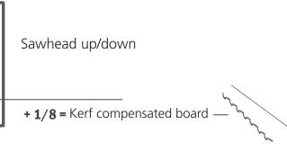
On the crank shaft, there is an opening where you can see numbers on a scale. This scale has eight steps, where each step is 1/8". **TIP:** When a board is cut above the blade, you have to compensate for the kerf, i.e. 1/8". The wood piece below the blade never needs to be kerf compensated. It has the same measurement that is shown on the absolute scale on the front leg of the carraige.
