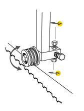
The blade guides must be adjusted so that they are parallel to the back of the blade. This is done by adjusting the outer and inner adjusting bolts. It is crucial that the blade guides run parallel to the blade. Be careful to adjust this correctly.
