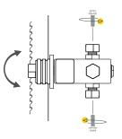
The blade guide can be adjusted inwards and outwards by pulling or pushing its shaft after the adjusting bolts have been loosened. The back of the blade should be approx. 3-5 mm from the rear edge of the blade guide roller.
