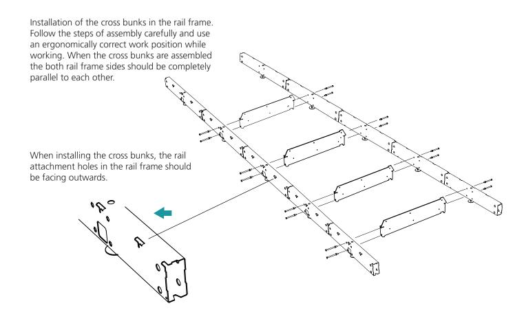
Prepare the bolt joints for the installation of the cross bunks in the rail frame. The nut should be tightened until there is 20 mm of free thread.
