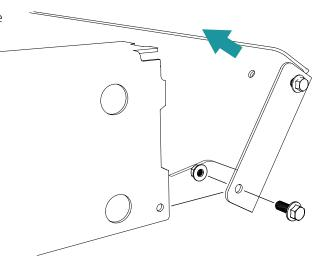
Prepare the bolt joints for the installation of the rail sections. Note that the flange nut should be fitted "backwards" on the bolt.
