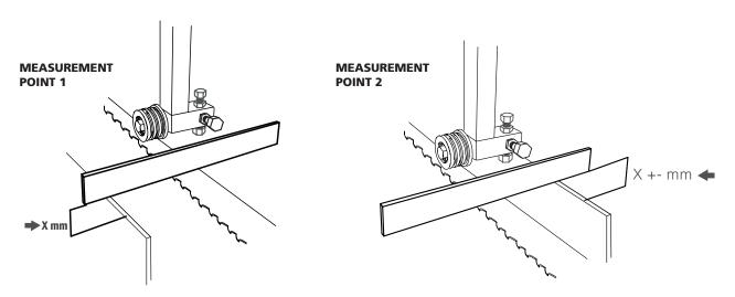
If the measurements differ, turn the adjusting bolts on the blade guide until the measurements are the same at both measurement points. One method to facilitate adjusting, is to use the value from measurement point 1, compare it with the value from measurement 2 and then, by raising or lowering the blade guide, adjust half the difference at measurement point 2. When the blade is parallel to the rails, repeat the adjustment steps on the other blade guide roller.
