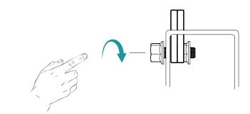
Tighten the bolt joints fingertight!
