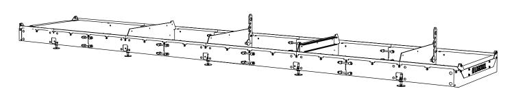
Fit the nut and the washer on the levelling foot.
