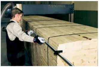
At the top and the bottom of both sides of the stack, set the stop plate against the cut surface and mark the end of the rod.
