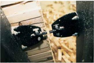
Once one of the stack's ends has been trimmed, the cut surface provides the point for measuring the position of the next cut.
