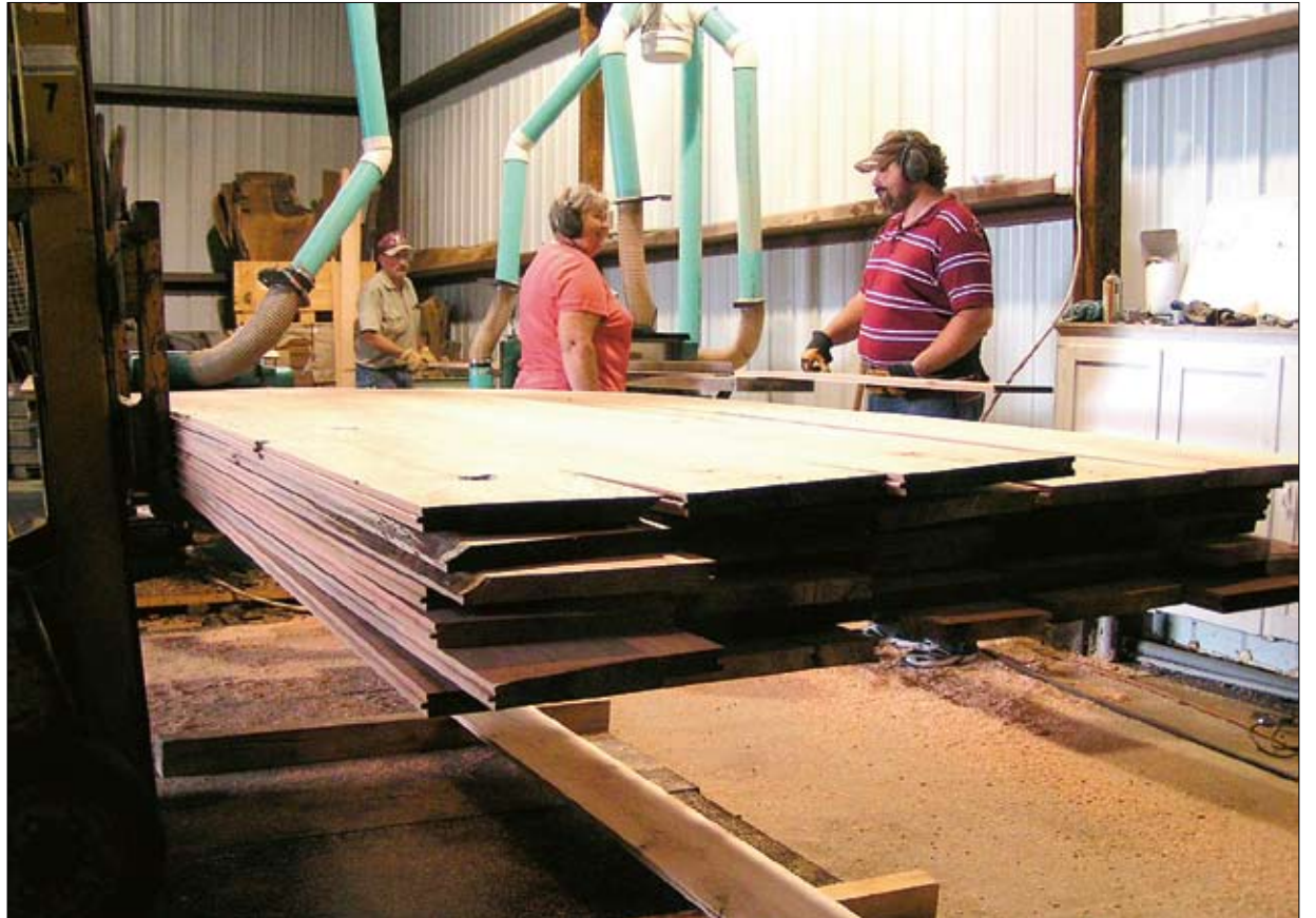
Ryan and Easter remove flooring from the PH260 while Steve feeds in the next rough board. After installation, they will need only a light sanding before finishing.
