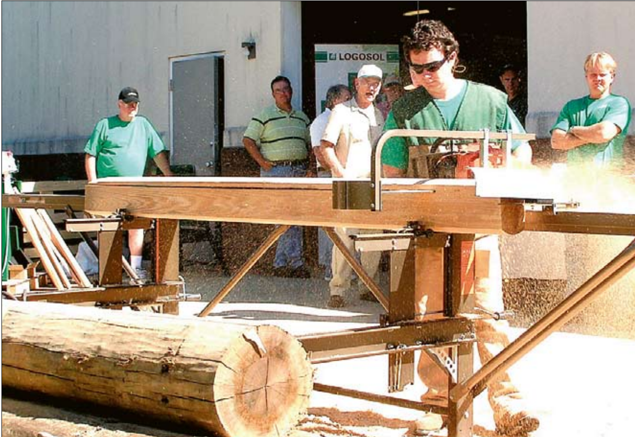
Rivers Griffin demonstrates how to use the M7 sawmill to make log house facing.
