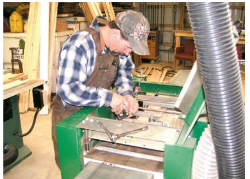
John Arnett installs a set of knives for a new trim pattern. He says it takes about thirty minutes to change the knives.
