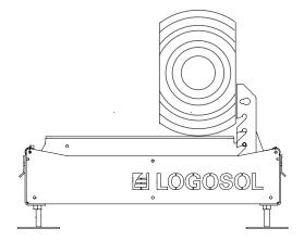
Rotate the log 90° so that one of the freshly sawn sides rests flat against the log supports, and then clamp the log in position.
