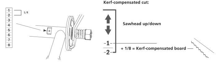
On the crank shaft, there is an opening where you can see numbers on a scale. This scale has eight steps, where each step is 1/8". **TIP:** When a board is cut above the blade, you have to compensate for the kerf, i.e. 1/8". The wood piece below the blade never needs to be kerf compensated. It has the same measurement that is shown on the absolute scale on the front leg of the carraige.
