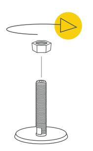
Install the leveling feet to the underside of the bed and secure with the lock nuts.
