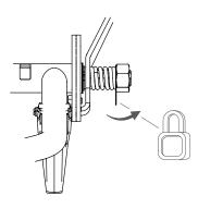
Once the handle is in good working order, you bend the lock washer to secure the lock nut in position.
