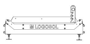
**3.** Use the accessory SMART Turner when rolling a log on the log bed. Centre the log on the log bed and roll it up against the log supports. Check the position of the log on the log bed. To be able to cut through the whole length of the log, the log should not protrude past the last cross bunk.
