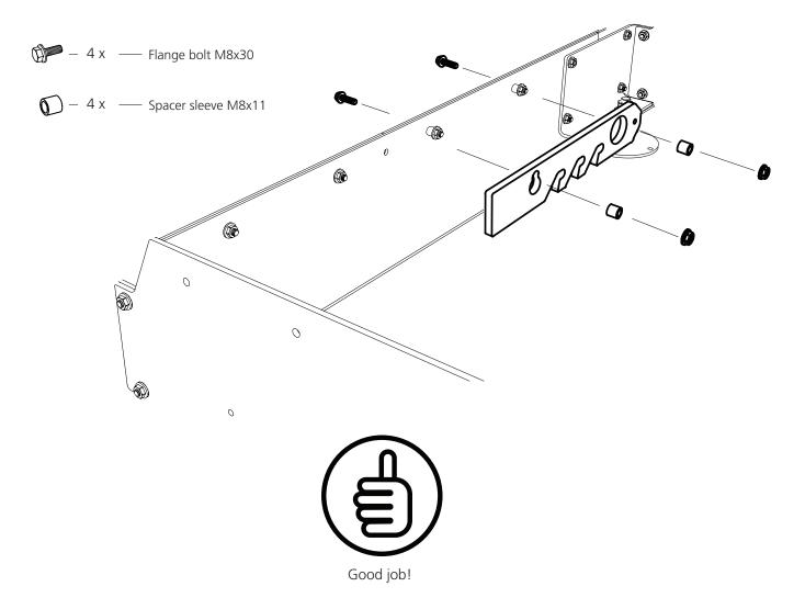
Now it is time to install the sawhead onto the rails.
