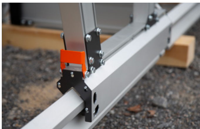
The saw carriage glides easily on the rail, completely free of play.
