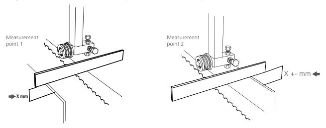
If the measurements differ, turn the adjusting bolts on the blade guide until the measurements are the same at both measurement points. One method to facilitate adjusting, is to use the value from measurement point 1, compare it with the value from measurement 2 and then, by raising or lowering the blade guide, adjust with half the difference at measurement point 2. When the blade is parallel to the rails, repeat the adjustment steps on the other blade guide roller.
