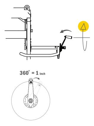
The locking mechanism of the crank is divided in eight steps per revolution. Each step moves the sawhead by 1/8", and one full revolution represents 1".
