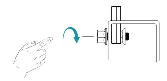
Tighten the bolt joints fingertight!
