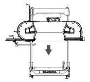
Tip: Work with the sawhead in its lowest position to facilitate access to the engine.
