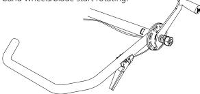
**13.** With both hands on the push handle, gently push the saw carriage forward until the blade begins to cut into the log. When the band blade is completely inside the log, you can increase the feed rate. Adjust the feed rate so the cut becomes straight with a clean finish. Lower the feed rate when cutting through knots in the wood and choose a lower speed when cutting large or hard logs. Also lower the feed rate when you come to the end of the log.
