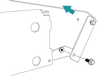
Prepare the bolt joints for the installation of the rail sections. Note that the flange nut should be fitted "backwards" on the bolt.
