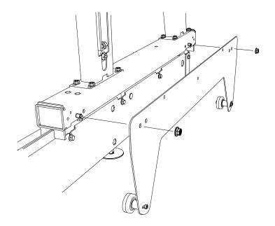
Fit the anti-tip plate to the bogie base. Repeat this on the other side of the machine.
