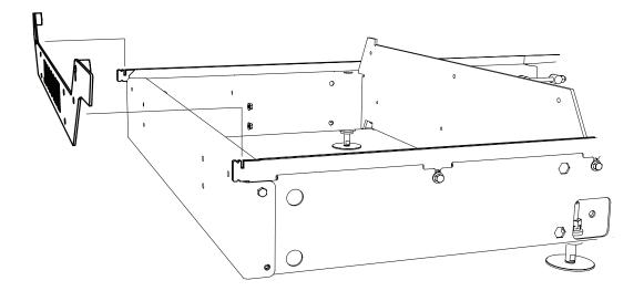
Secure the outer end plates with bolts and nuts.
