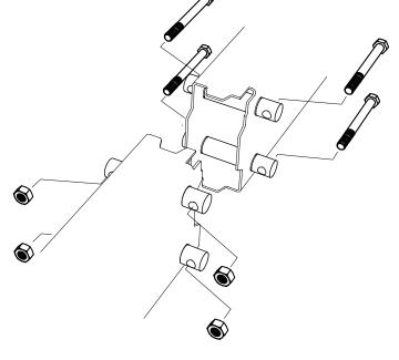
Secure the bolt joints. Ensure that the joint between the rail frame sections stays straight when tightening the bolt joints.
