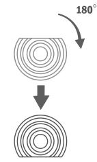
Rotate the log 180° so that the freshly sawn surface rests on the log bed.
