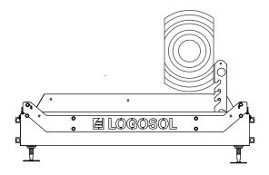
Rotate the log 90° so that one of the freshly sawn sides rests flat against the log supports, and then clamp the log in position.
