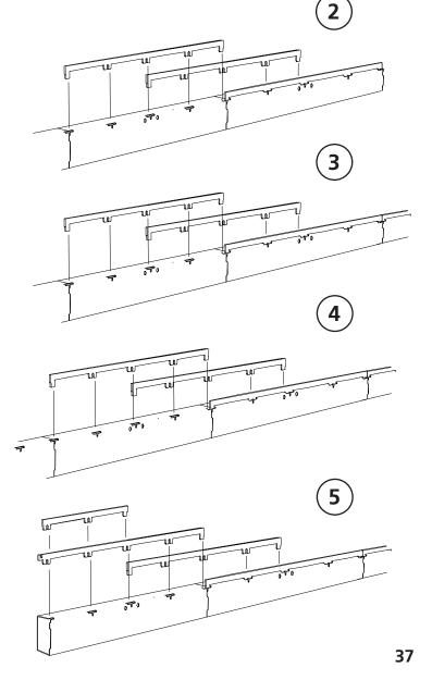
The last short rail section should be fitted the same way as the first one. See the first step of assembly on page 36.
