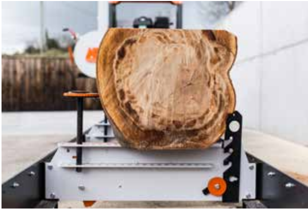
• Reliable rail frame remains straight even under the load of the heaviest logs
