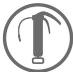
When this symbol appears during assembly, parts must be lubricated before installation. Lubricate affected parts with universal grease.
