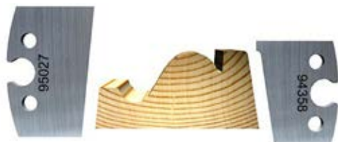
Lower window lining
