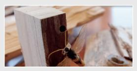
• Wood wasp larvae survive sawing and drying.
